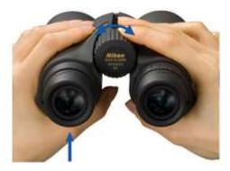
Next, look at the same object through the right eyepiece with your right eye (left eye closed). Rotate the diopter adjustment ring (usually located on the right eyepiece) until you see a sharp image.
