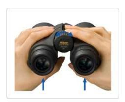
Looking through both eyepieces, focus on an object by rotating the focusing ring. If the diopter has been adjusted, turn *only* the focusing ring to focus whenever you change the object viewed.
