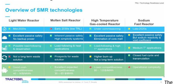
Light Water reactors use current **GenIII** nuclear technology while the last three use **GenIV** technology
